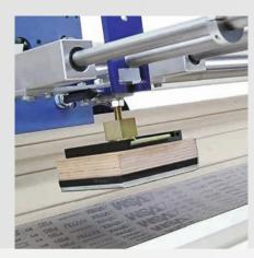
Grinding pad with ball-type quick fastener.
