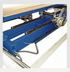
3D handling unit can be moved on guides from the centre to the right side of the table.
