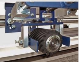
Grinding unit with quick change system for contact rollers and grinding pads.
