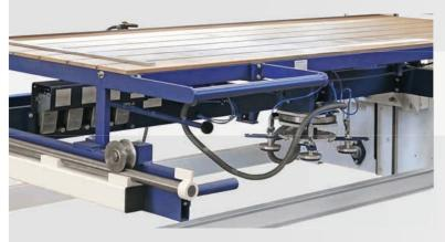
Flat machine table as an add-on table. The 3D handling device pivoted downwards and stored underneath.
