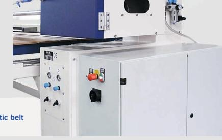
Right-hand machine stand with offset, switches and pressure regulator for pneumatic belt tensioning. Operated from the front.
