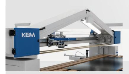
The grinding unit is mounted on a stable guide and is driven via a timing belt. The contact roller automatically moves between the two grinding belts, depending on the selected grinding program.
