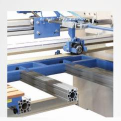
Aluminium cantilever arms to hold box-shaped workpieces.
