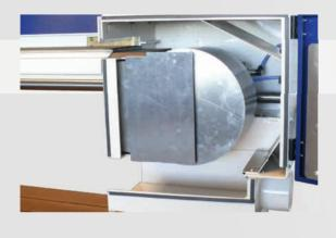
Grinding unit with grinding pad equipped with a ball quick clamp. Optionally available with a grinding roller. Idle pully and roller cover made of aluminum to prevent dust deposits in the idle pully.
