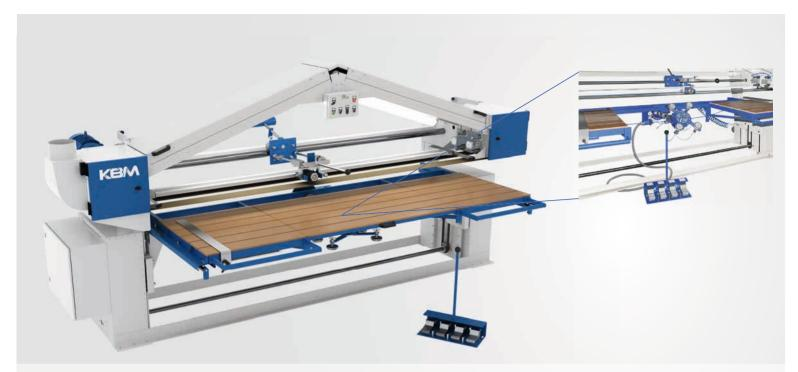
The handling device is mounted in the centre of the table beneath the insertion frame. The rotating and pivoting axes are unlocked pneumatically by foot switches; the rotary axes are moved manually.
