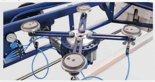
The device is equipped with four vacuum suction cups for holding the workpieces. The pivoting mechanism can be locked at  $0^{\circ}$ ,  $22.5^{\circ}$ ,  $45^{\circ}$ ,  $67.5^{\circ}$  and  $90^{\circ}$ .
