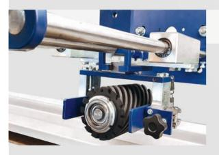
Grinding unit with quick change system for contact rollers and grinding pads.
